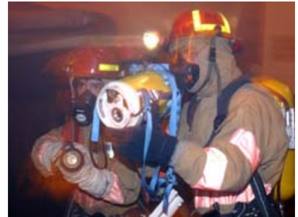
EEV P4428 NFTI, the original Navy Firefighting Imager
