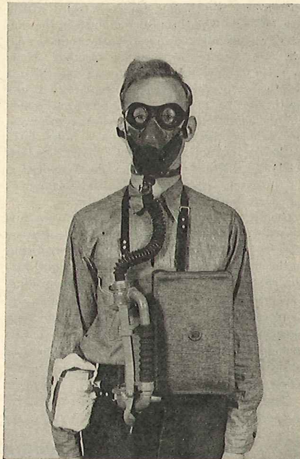
FIGURE 2—Front view, facepiece valve depressed permitting wearer to breathe from surrounding atmosphere.
