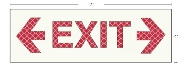
DAMAGE CONTROL SIGNAGE SKETCH # 045 EXIT (12" x 4" left arrow), (12" x 4" right arrow) and (12" x 4" double arrow)
