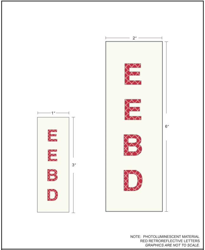
**DAMAGE CONTROL SIGNAGE SKETCH # 039** EEBD (1" x 3" vertical) and (2" x 6" vertical)
