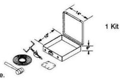
Helpful Hints: Current requirement - stow items together as kit in DCRS. Requirement is for two 100 foot rolls of 1/2" steel strapping and one box containing (100) 1/2" seals (buckles) for steel strapping, clamping tool and a ball peen hammer.
