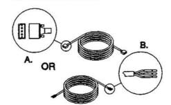
Helpful Hints: Only 1 casualty power cable required per DCRS. It should be stowed in P-way and identified for DCRS & length at the stowage rack label plate.
