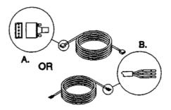
Helpful Hints: Only 1 casualty power cable required per DCRS. It should be stowed in P-way and identified for DCRS & length at the stowage rack label plate.
