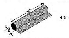
Helpful Hints: Used to cut gaskets for backside of strongbacks in banding kit and jubilee patches, box patches and soft patches in the pipe patching kit.
