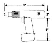
Helpful Hints: Removable energy pack, reversible, high torque. Used for drilling pilot holes, driving lag bolts and self tapping screws.
