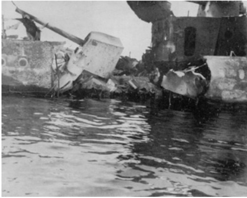
Photo 5: USS ERIE - Beached. Torpedo Damage, starboard quarter.
